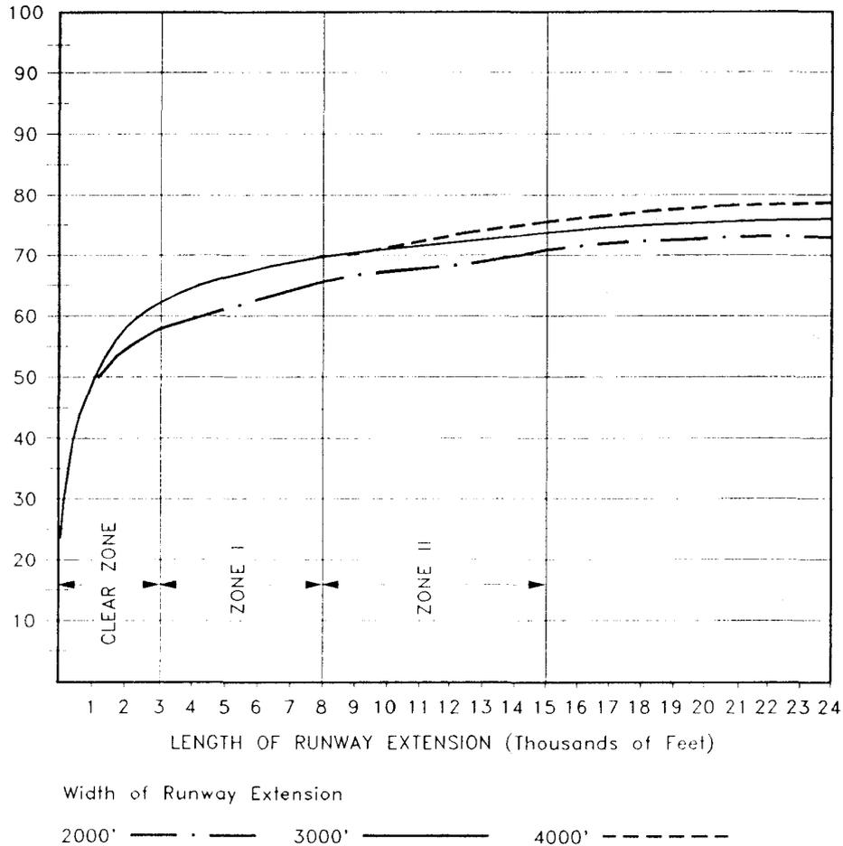
Using the optimum runway extension width, 3,000 feet, and the cumulative distribution of accidents from the end of the runway, zones were established which minimized the land area included and maximized the percentage of accidents included. The zone dimensions and accident statistics for the 1968-1972 study are shown in Figure B-2.
